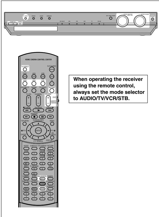
When operating the receiver using the remote control, always set the mode selector to AUDIO/TV/VCR/STB.
