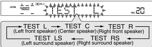
**4 Adjust the following speaker output levels (from -10 dB to +10 dB).**
