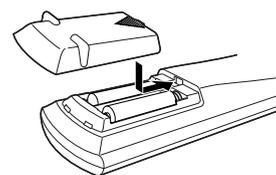
If the range or effectiveness of the remote control decreases, replace the batteries. Use two R6P(SUM-3)/AA(15F) type dry-cell batteries.
