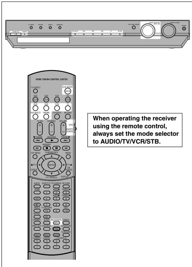
When operating the receiver using the remote control, always set the mode selector to AUDIO/TV/VCR/STB.
