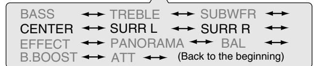
**CENTER\*:** To adjust the center speaker output level (from -10 dB to +10 dB).
