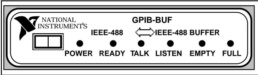
Figure 1-2. The GPIB-BUF Front Panel
