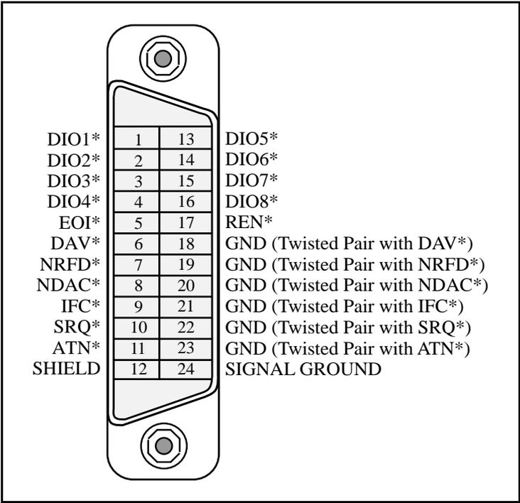
Figure 1-4. The GPIB Connector and Signal Designations
