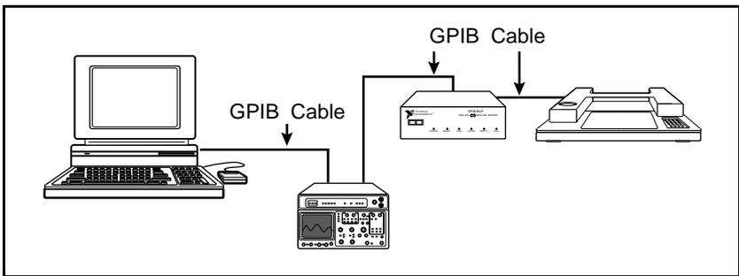
Figure 2-1. GPIB-BUF System Setup Example
