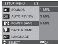
**1/3/5 MIN** The camera is designed to switch off automatically to save battery life after the specified period of inactivity.
