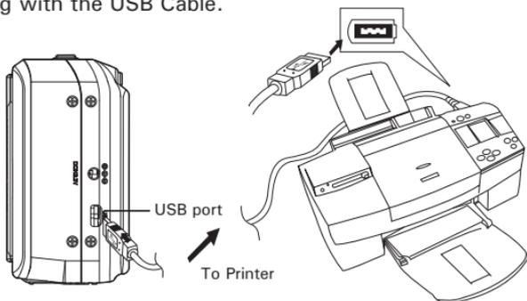
1. Plug the labelled end
