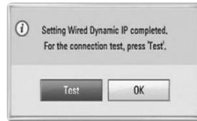
5. If you select [Test] and press ENTER (Ⓢ) at step 4 above, the network connection status is displayed on the screen. You can also test it on the [Connection Status] in the [Setup] menu.
