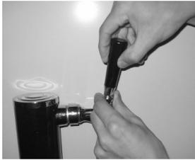
Attach the black plastic lever (pull handle) provided on the top of the faucet tightening it by hand clockwise until the end, holding in the silver snug underneath so it does not move.
