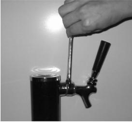
Spanner faucet wrench provided for either removing or tightening connection
