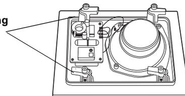
To remove the speaker from the wall or ceiling, loosen the screws only far enough to remove the speaker. This will prevent loss of the mounting tabs.
