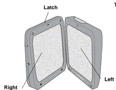
1. While holding the latch on the top of the right speaker, pull the speaker halves apart to separate them.
