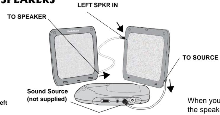
4. Pull out **TO SOURCE** (the right speaker's 1/8-inch stereo plug) until it stops, then insert it into your sound source's audio output or headphone jack. Then pull out **TO SPEAKER** (the left speaker's 1/8-inch mono plug) until it stops. Then insert it into **LEFT SPKR IN** on the right speaker.
