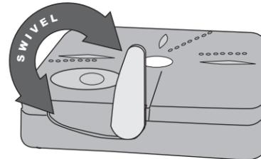
2. Rotate the stand on the bottom of both speakers. Then place both speakers on a level surface.
