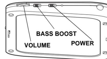
3. On the right speaker, set **POWER** to **OFF** and rotate **VOLUME** to its minimum position until it stops.
