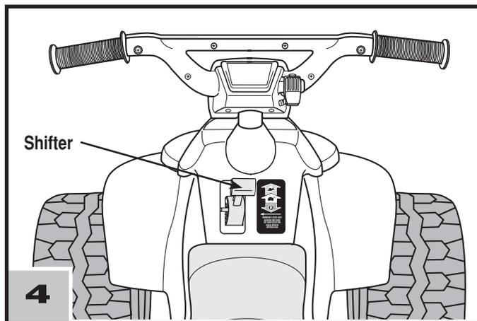
**IMPORTANT!** To avoid damaging the motors and gears, stop the vehicle before shifting between low and high speed.
