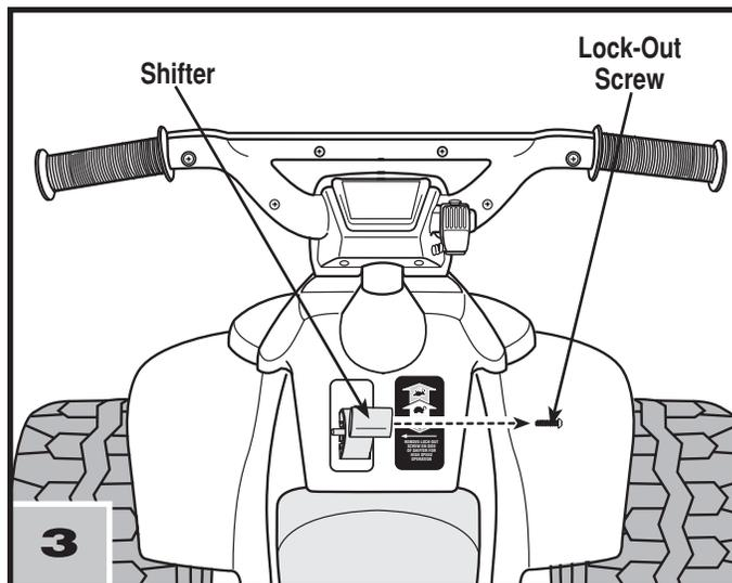
**Before you disconnect the high speed lock-out**, make sure your child knows how to start and stop the vehicle and knows the rules for safe driving. When the high speed lock-out is removed, the vehicle can be driven forward in low speed (2½ mph, maximum) or high speed (5 mph, maximum).
