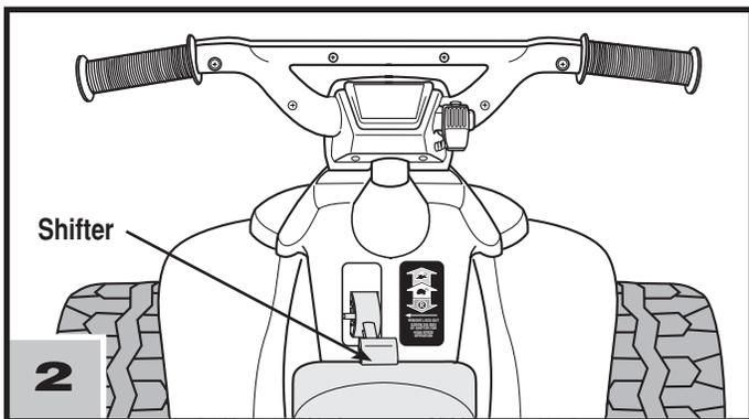
**IMPORTANT!** To avoid damaging the motors and gears, make sure to stop the vehicle before switching from forward to reverse.
