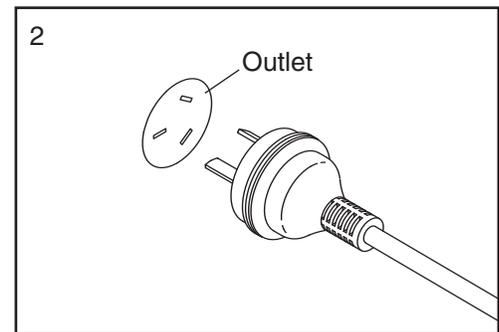
**⚠ DANGER:** Improper connection of the equipment-earthing conductor can result in an increased risk of electric shock. Check with a qualified electrician or serviceman if you are in doubt as to whether the product is properly earthed. Do not modify the plug provided with the product—if it will not fit the outlet, have a proper outlet installed by a qualified electrician.
