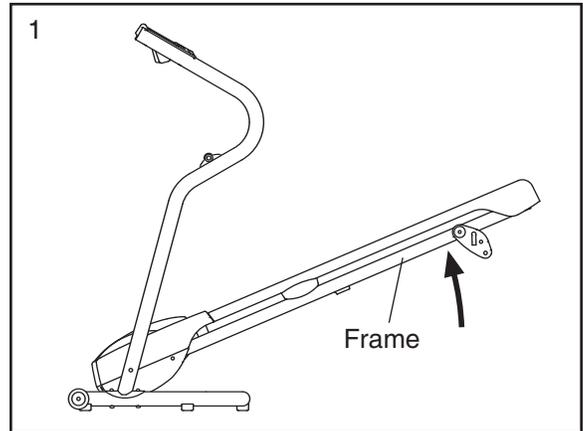
2. Move your right hand to the position shown and hold the treadmill firmly. Using your left hand, pull the latch knob to the left and hold it. Raise the frame until the hole in the catch is aligned with the latch pin. Slowly release the latch knob; **make sure that the latch pin is fully inserted into the catch.**
