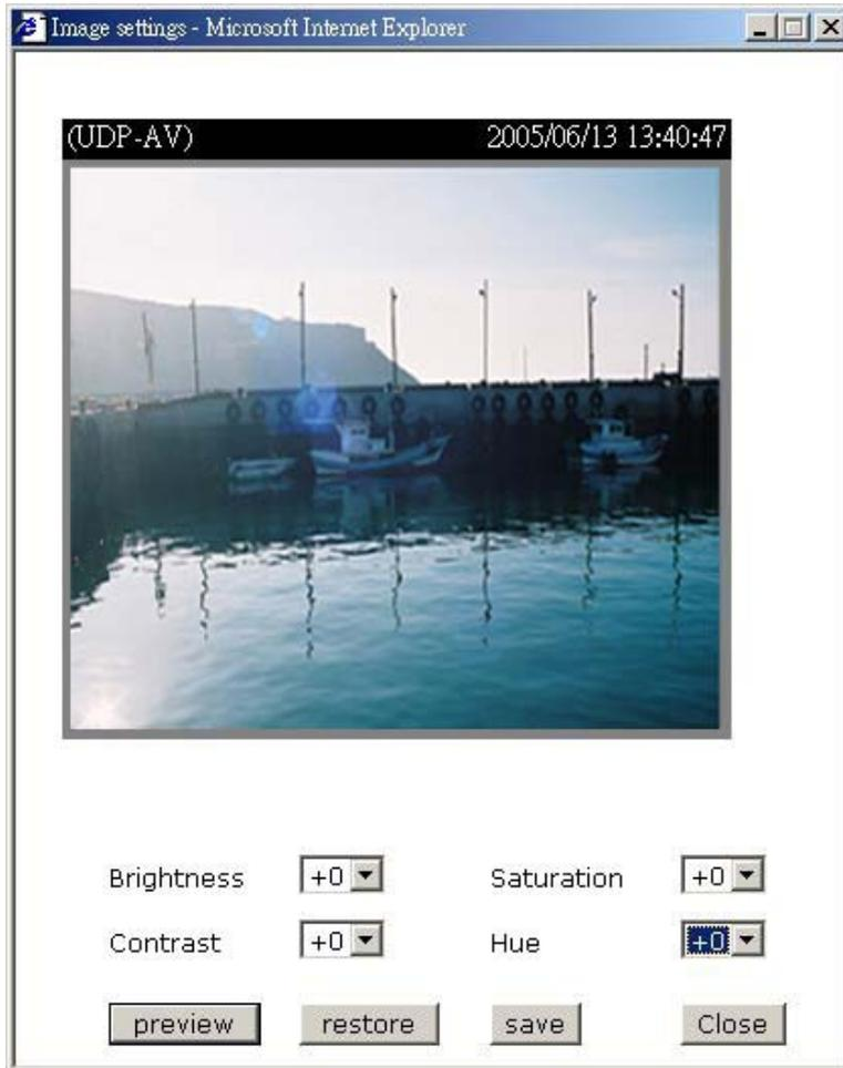
levels ranged from -5 to +5. In **“Brightness”** and **“Contrast”** fields the value 0 indicates auto tuning. The user may press **Preview** to fine-tune the image. When the image is O.K., press **Save** to set the image settings. **Restore** Click on this to recall the original settings without incorporating the changes.
