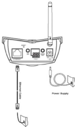
Please verify that your product package contains all the accessories listed in the foregoing Package Contents. Depending on the user's application, an Ethernet cable may be needed. The Ethernet cable should meet the specs of UTP Category 5 and not exceed 100 meters in length.
