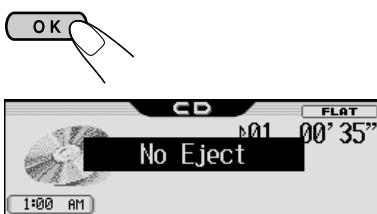
“No Eject” flashes, and the disc cannot be ejected.
