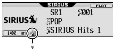
\* Signal strength bar increases as the receiving signal improves. If no signal is received, it disappear.
