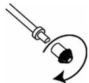
**13** Restore the center shaft with center gear into the original position and rotate center gear so the front center gear meshes with the shaft.
