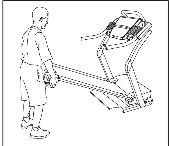
2. Move your right hand to the position shown and hold the treadmill firmly. Pull the latch knob to the left and hold it. Raise the treadmill until the platform passes the pin on the latch knob. Release the latch knob. **Make sure that the plate is resting against the pin as shown.**
