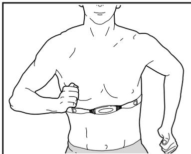
Pull the sensor unit away from your body a few inches and locate the two electrode areas on the inner side (the electrode areas are covered by shallow ridges). Using saline solution such as saliva or contact lens solution, wet both electrode areas. Return the sensor unit to a position against your chest.
