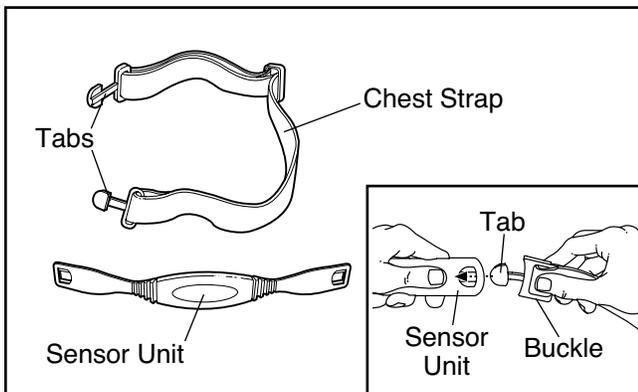
Next, wrap the chest pulse sensor around your chest and attach the other end of the chest strap to the sensor unit. Adjust the length of the chest strap, if necessary. The chest pulse sensor should be under your clothes, tight against your skin, and as high under the pectoral muscles or breasts as is comfortable. Make sure that the logo on the sensor unit is facing forward and is right-side-up.
