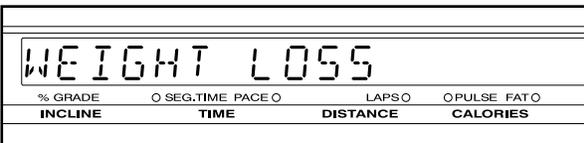
Next, press the Select Course button repeatedly to select one of the weight loss, aerobic, or performance programs. For example, if the words “WEIGHT LOSS” appear in the main display, you can select the 20-minute Pyramid, 35-minute Pyramid, 20-minute Fat Burn, or 20-minute Interval program.
