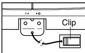
Test the clip by carefully taking a few steps backward until the key is pulled from the console. If the key is not pulled from the console, adjust the position of the clip as needed. Then, remove the key from the console.
