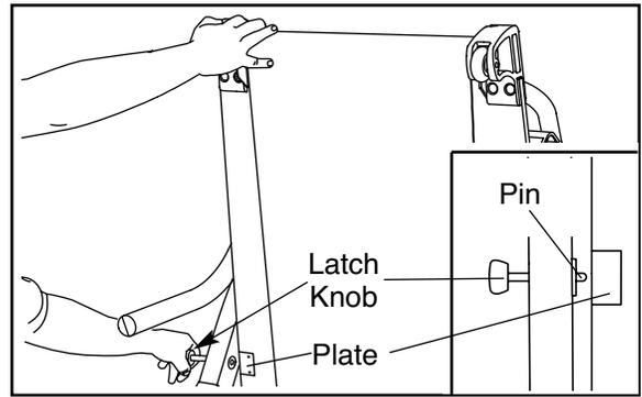
2. Hold the treadmill firmly with both hands, and lower the treadmill to the floor. **Do not drop the treadmill frame to the floor. CAUTION: To decrease the possibility of injury, bend your legs and keep your back straight.**
