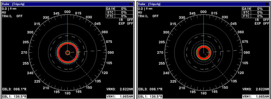
**Before adjusting the Trigger Delay for 4 kW radars, two rings will be shown on the screen (left). As Trigger Delay is increased, the larger ring will start to get smaller. The small ring will disappear (right).**
