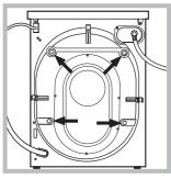
3. Remove the 4 protective screws and the rubber bush with the respective spacer, situated on the rear of the appliance (see also the installation leaflet). NB:The plastic spacers may fall down inside the machine once the bolt
