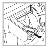
Remove the dispenser by raising it and pulling it out (see figure). Wash it under running water; this operation should be repeated frequently.
