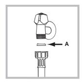
1. Insert seal A into the end of the inlet hose and screw the latter onto a cold water tap with a 3/4 gas threaded mouth (see figure).
