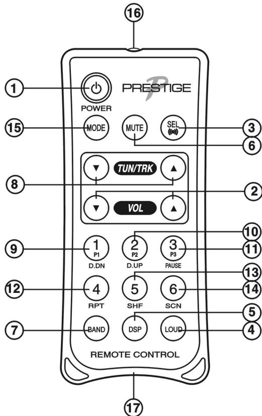
The wireless remote control supplied with this model is capable of operating most of the features of the unit from a remote location. Each button on the remote control functions in the same way as the referenced button on the main unit. For optimal operation of the remote control, always aim it toward the Remote Sensor ⑳ on the front panel of the main unit.
