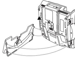
3. Align the bracket's keyhole slots with the screws, then slide the base downward to secure it.
