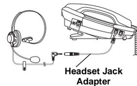
To connect the headset with a sub-mini plug, first plug the supplied headset jack adapter (sub-mini to modular converter) into the modular
