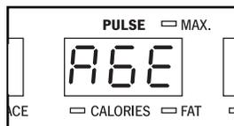
After you have entered your age, the letters "SPd" and the maximum speed setting of the program will flash in the Pulse/Calories/Fat Calories display. If desired, press the  $\Delta$  and  $\nabla$  buttons beside the Enter button to adjust the maximum speed setting. When the desired setting is shown, press the Enter button.
