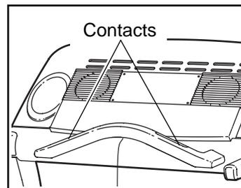
metal contacts on the handgrip pulse sensor. Your palms should be resting on the upper contacts. **Avoid moving your hands.** When your pulse is detected, two dashes (--) will appear in the Pulse/Calories/Fat Calories display, and then your heart rate will be shown. **For the most accurate heart rate reading, continue to hold the contacts for about 15 seconds.**
