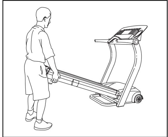
2. Hold the treadmill firmly with your left hand. Using your right hand, pull the lock knob to the right and hold it. Raise the treadmill until the pin on the lock knob is aligned with the hole in the left foam grip. Then, release the lock knob. **Make sure that the lock knob is fully released so the pin is fully inserted into the hole in the left foam grip.**
