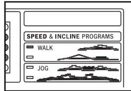
When a preset workout program is selected, the Distance/Incline/Laps display will flash the maximum incline setting of the program, and the Speed display will flash the maximum speed setting, for six seconds. The Time/Segment Time/Pace display will show how long the program will last.
