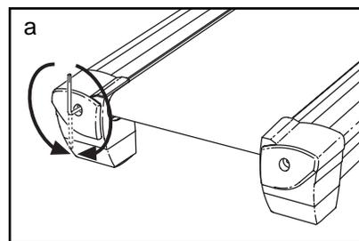
b. If the walking belt slips when walked on, first remove the key and **UNPLUG THE POWER CORD**. Using the allen wrench, turn both rear roller bolts clockwise 1/4 of a turn. When the walking belt is correctly tightened, you should be able to lift each side of the walking belt 3 to 4 inches off the walking platform. Be careful to keep the walking belt centered. Plug in the power cord, insert the key, and walk on the treadmill for a few minutes. Repeat until the walking belt is properly tightened.
