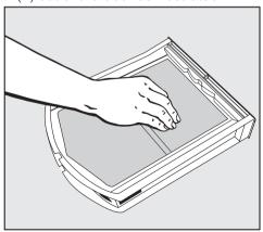
■ Use your fingers to remove the fluff from the surface of the filter
