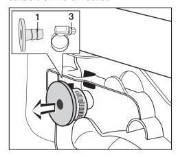
Remove the following from the back of the dryer at the top: Adapter 1 and hose clip 3 behind it.
