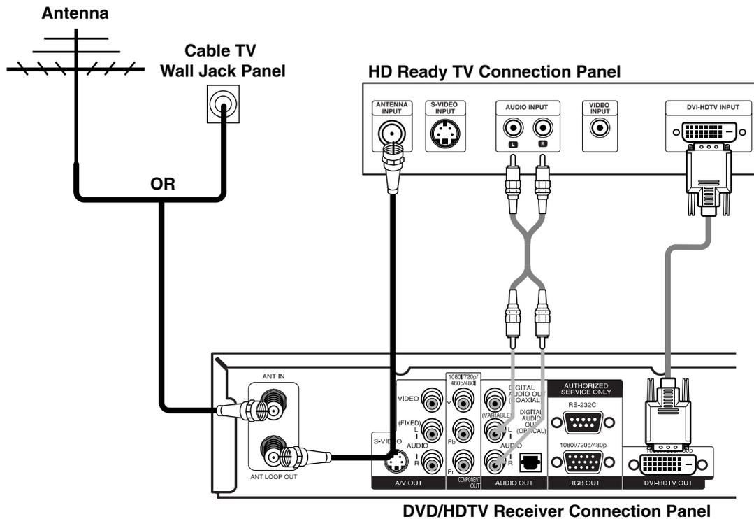
**1** Connect the “Antenna/Cable” to the “ANT IN” jack on the DVD/HDTV Receiver using a coaxial RF cable.
