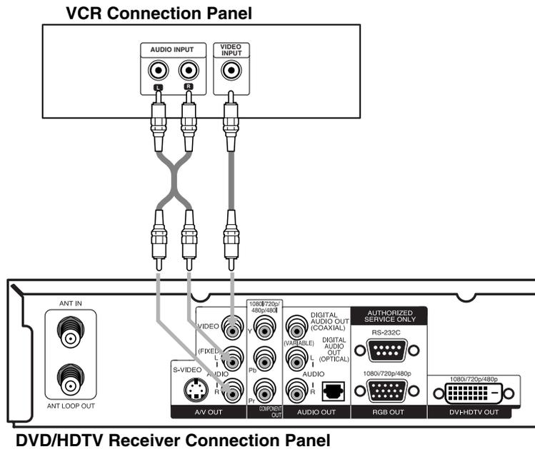
Connect the L/R “AUDIO OUT” jacks and “VIDEO OUT” jack on the DVD/HDTV Receiver to the “A/V in” jacks on your VCR using RCA-type cables. (If your VCR is equipped with an S-Video jack, use the “S-Video” jack.)
