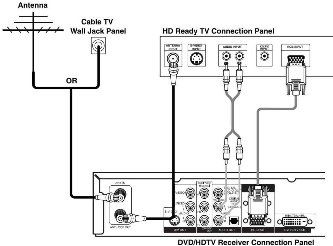
**1** Connect the “Antenna/Cable” to the “ANT IN” jack on the DVD/HDTV Receiver using a coaxial RF cable.
