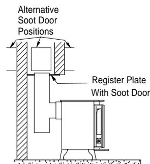
Fig. 5. Horizontal Register Plate With Rear Flue Connection
