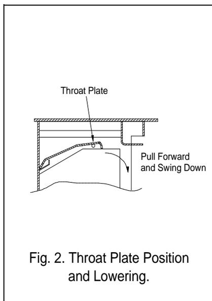
Fig. 2. Throat Plate Position and Lowering.
