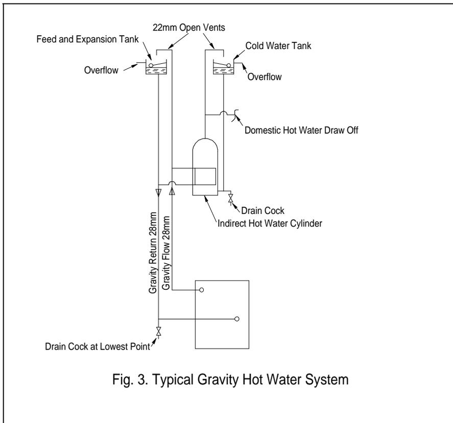
Fig. 3. Typical Gravity Hot Water System
