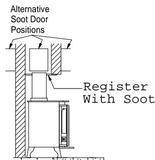
Fig. 6. Horizontal Register Plate With Top Flue Connection
