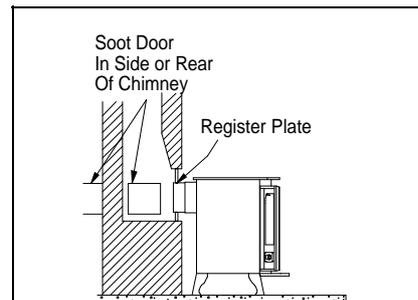
Fig. 4. Vertical Register Plate With Bricked Up Fireplace
