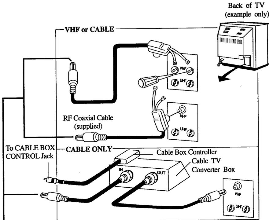
*If you have a UHF-only antenna system: Even if you only plan to play tapes and view/record UHF channels, you still need to make one of the combination UHF/VHF connections shown above. This is because when your VCR operates, it sends VHF signals to the TV across the RF coaxial cable.*
