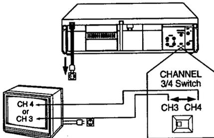
**1** Set the TV to channel 3 or 4, whichever channel the CH3/CH4 switch on the back of the TV is set to.
