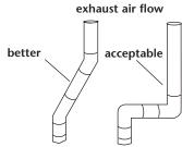
Select the route that will provide the straightest and most direct path outdoors. Plan the installation to use the fewest number of elbows and turns.
