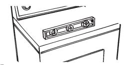
Check levelness of dryer by placing a level on top of dryer, first side to side, then front to back. If dryer is not level, adjust dryer legs up or down.
