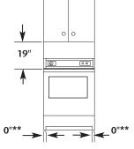
\*\* Wall, door and floor molding may require additional spacing.
