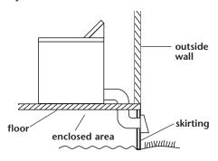
The exhaust vent must be securely fastened to a non-combustible portion of the mobile home structure. The exhaust system must not terminate beneath the mobile home.
