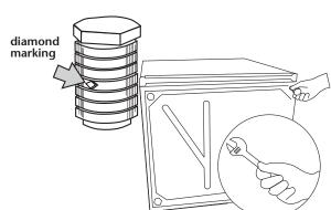
Start to screw legs into holes by hand. Use an adjustable wrench or 1" hex-head socket wrench to finish turning legs until you reach the ridge with the diamond marking.
