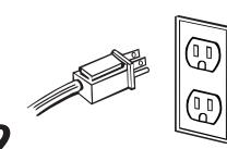
Plug power supply cord into grounded 3-prong outlet.
