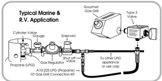
**IMPORTANT!! ■ DO NOT CONNECT A HIGH-PRESSURE SUPPLY HOSE FROM A NON-REGULATED TANK DIRECTLY TO GRILL.**
