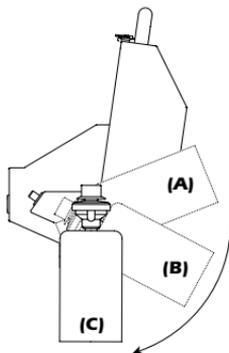
**Valve will feel loose and will rotate easily. Even though the valve feels loose, it will not leak. The valve was designed to be loose fitting in order to allow safe, easy installation and removal of the propane canister and so it easily swings without resistance to fit all applications.**
