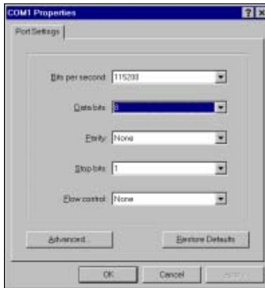
Figure 7-1 Serial port settings.
