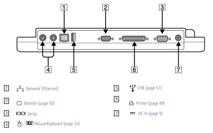
The port replicator can be powered only with an AC power adapter. Do not remove the AC adapter from the port replicator or the AC outlet while using the port replicator; this may cause data damage or hardware malfunctions.
