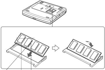
1 Slide the memory module into the slot.
