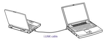
i.LINK cables compatible with your VAIO notebook include cables with the following part numbers: VMC-IL4415 (a 1.5-meter cable with a 4-pin connector at each end), VMC-IL4615 (a 1.5 meter-cable with a 4-pin connector at one end and a 6-pin connector at the other), and VMC-IL4408A (a 0.8-meter cable with a 4-pin connector at each end).
