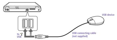
You can use the optional Sony USB mouse PCGA-UMS1 with this computer. The USB mouse software driver is preinstalled in the computer. Therefore, you only need to plug the USB mouse into the USB connector.
