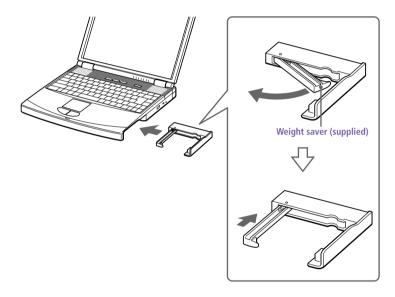
3 Manually lock the weight saver's Release lever.
