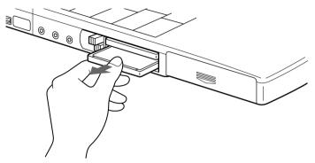
Insert the PC card into the PC card slot, front label facing up. Gently push the card into the slot until the card is fixed into the connector. The release button comes out.
