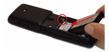
**3** Insert battery with the label readable. Align the contacts of the battery with the corresponding connectors on the battery compartment and insert in the direction of the arrow.
