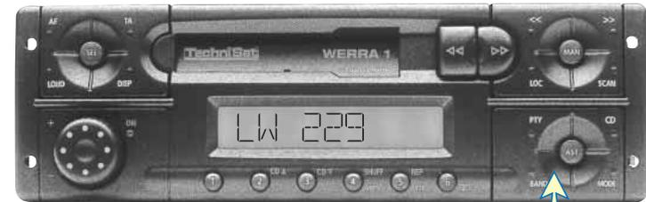
Step 1: Push for approx. 2 sec.; select the AM band; switch between MW, LW and SW by shortly pushing this button
