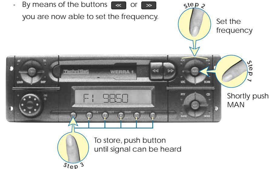
A short push on the respective button will change the frequency by 0.05 MHz; when the button is pushed and held for a longer time the frequency runs until the button is released.
