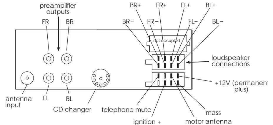
If your car does not have these connection possibilities you can also connect the device as follows. In that case, the ON/OFF switching function via the ignition lock is not activated. The same applies to the security LED.
