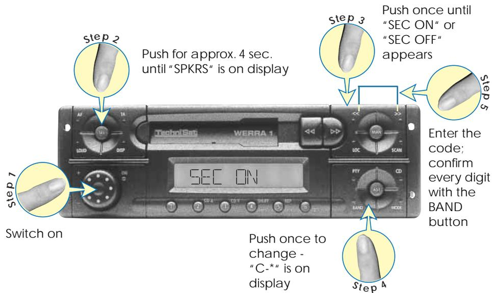
If you have entered a wrong code the device will switch off after a few seconds. The message "SEC ERR" is now shown on the display. Afterwards the code has to be re-entered.
