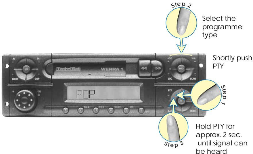
The TechniSat WERRA 1 is now searching for a station with the same programme type. It stops on the first station which corresponds to the selected programme type.
