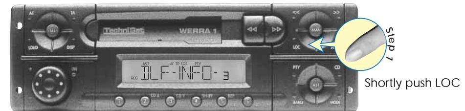
When set to "local" the automatic station search stops only at stations which can strongly be received. If no station can be found the function will automatically switch to normal searching sensitivity.
