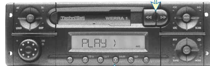
Shortly push button 4 to switch on the AMS mode; push again to switch it off
