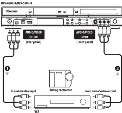
**1 Connect a set of audio and video inputs of your VCR or camcorder to a set of outputs on this recorder.**
