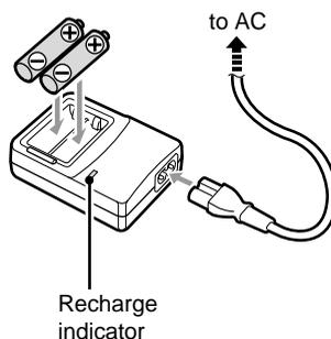
Recharge time of the supplied nickel metal hydride batteries: approx. 200 minutes for two batteries.
