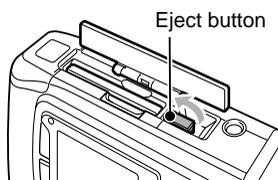
**5** Push in the eject button and remove the card.
