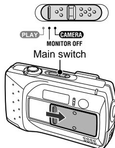
**3** Make sure the accessing indicator is not flashing, then open the card slot cover on the bottom of the digital camera.
