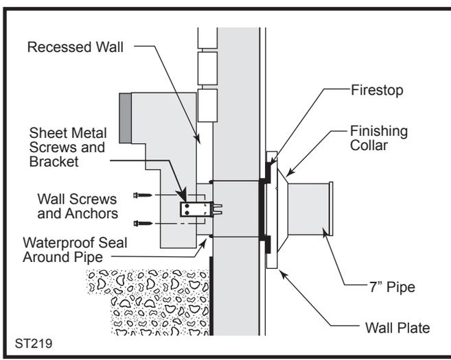
**Fig. 30** Use extension brackets to mount snorkel against recessed wall.
