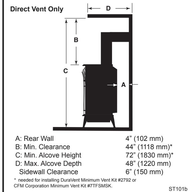
**Fig. 6** Dimensions and clearances to ceiling or alcove.
