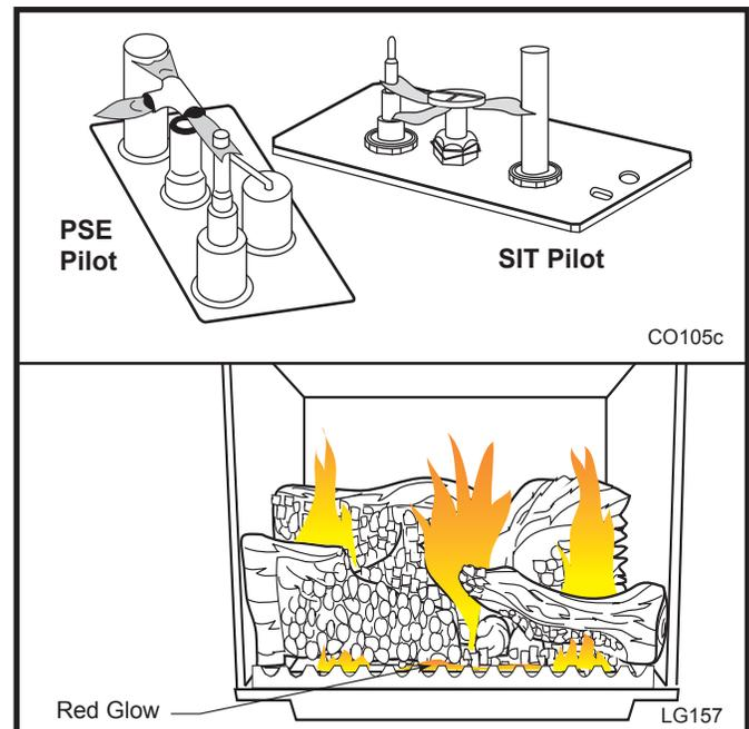
Fig. 48 Correct pilot and burner flame patterns.
