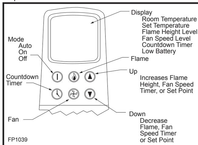
Fig. 50 Transmitter diagram.
