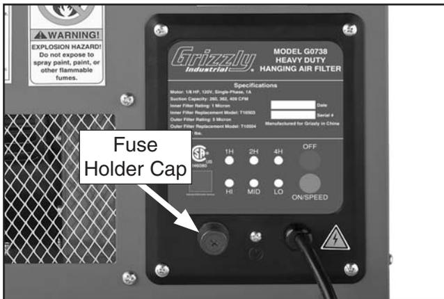
**Figure 16.** Fuse holder cap on the control panel.
