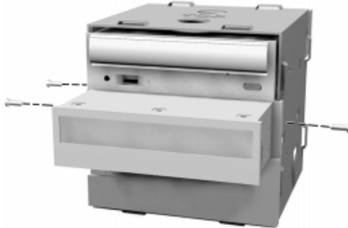
4. Slide the device out from the front of the system unit.
