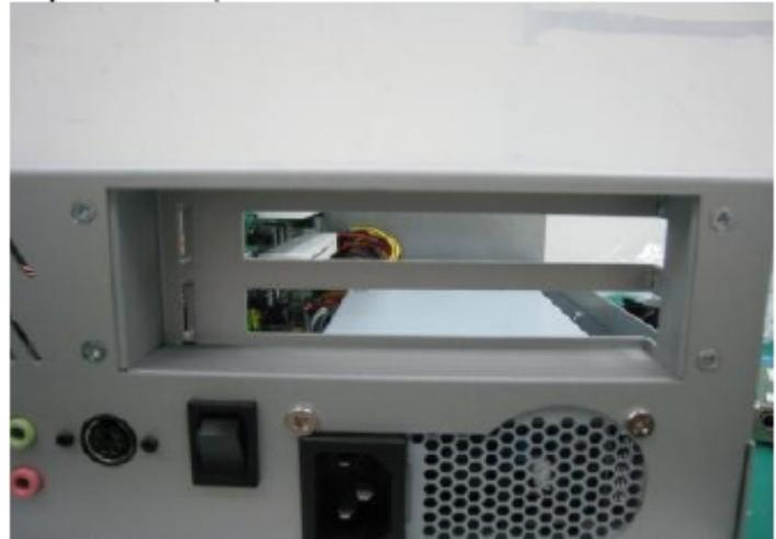
Step 4: Insert the add-on card in the socket firmly until it is completely sealed.
