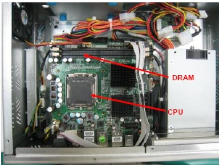
Step 3: Install the CPU and DDR DRAM in the PC 8120.
