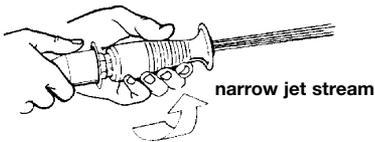
For low pressure operation, extend the nozzle of the multi-adjustable spray wand as shown.
