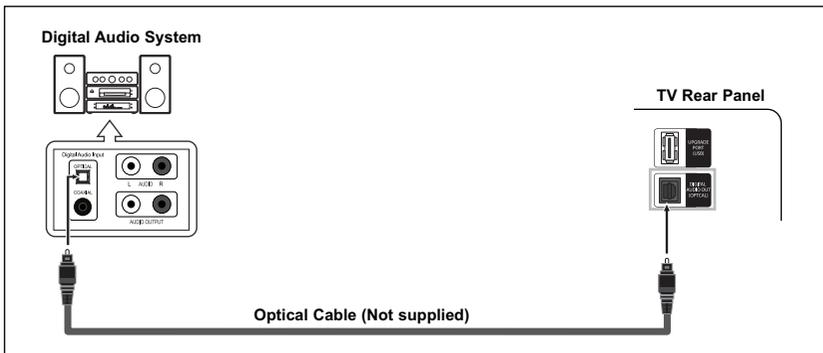
1. Connect an Optical Cable between the [DIGITAL AUDIO OUT (OPTICAL)] jacks on the TV and the Digital Audio Input jacks on the Digital Audio System.
