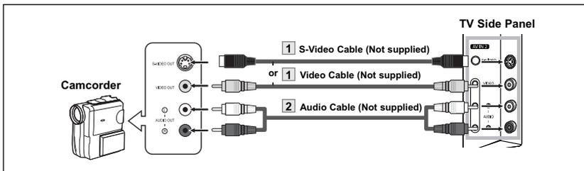
1. Connect a Video Cable (or S-Video Cable) between the AV IN2 [VIDEO] (or S-VIDEO) jack on the TV and the VIDEO OUT jack on the camcorder.
