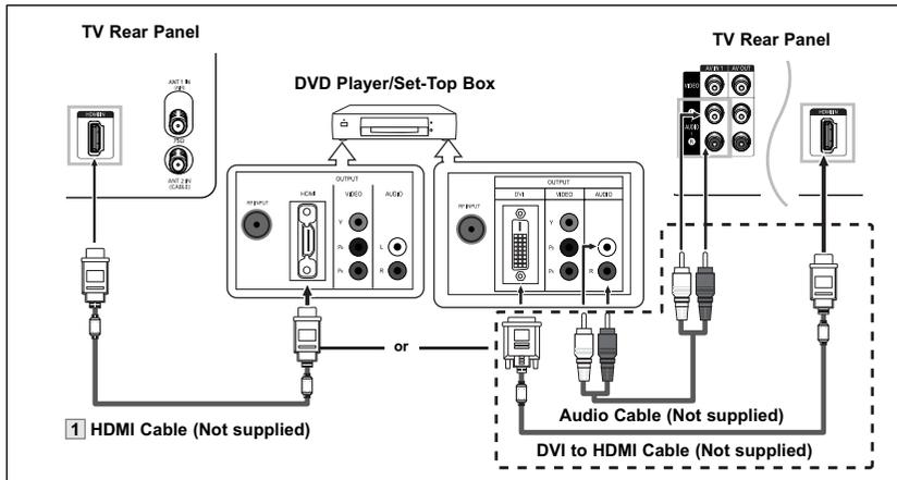
1. Connect an HDMI Cable between the [HDMI IN] on the TV and the HDMI OUT on the DVD player/Set-Top Box or connect a DVI to HDMI Cable or DVI-HDMI Adapter between the [HDMI IN] jack on the TV and the DVI jack on the DVD player/Set-Top Box.
