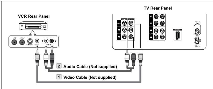
1. Connect a video cable between the AV OUT [VIDEO] jack on the TV and the VIDEO IN jack on the VCR. Refer to your VCR's instructions for more information about how to record using this kind of connection.
