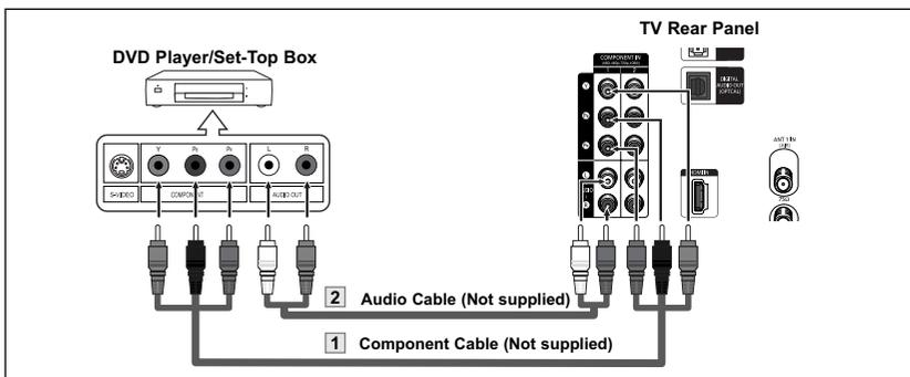
1. Connect a Component Cable between the COMPONENT IN 1 [Y, PB, PR] (or COMPONENT IN 2 [Y, PB, PR]) jacks on the TV and the COMPONENT Y, PB, PR jacks on the DVD Player/Set-Top Box.
