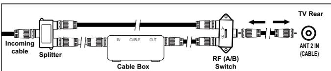
6. Connect the last Antenna cable between the OUT terminal on the RF (A/B) switch and the ANT 2 IN (CABLE) terminal on the back of the TV.
