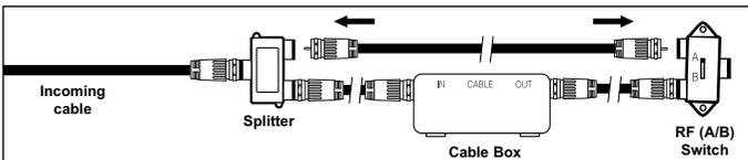
5. Connect another cable between the other OUT terminal on the splitter and the A-IN terminal on the RF (A/B) switch.
