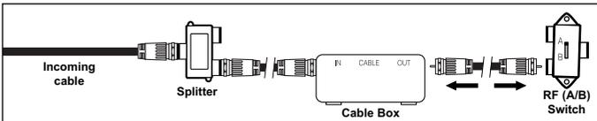
4. Connect an Antenna cable between the ANT OUT terminal on the cable box and the B-IN terminal on the RF (A/B) switch.
