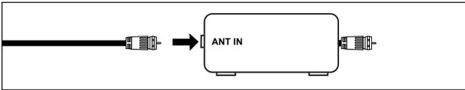
1. Find and disconnect the cable that is connected to the ANT IN terminal on your cable box.
