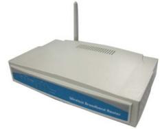
Plus, with the LAN DHCP feature, the WBR480 automatically completes the network configuration on itself and on all computers connected to the local area network. Zero configuration effort is needed for users.
