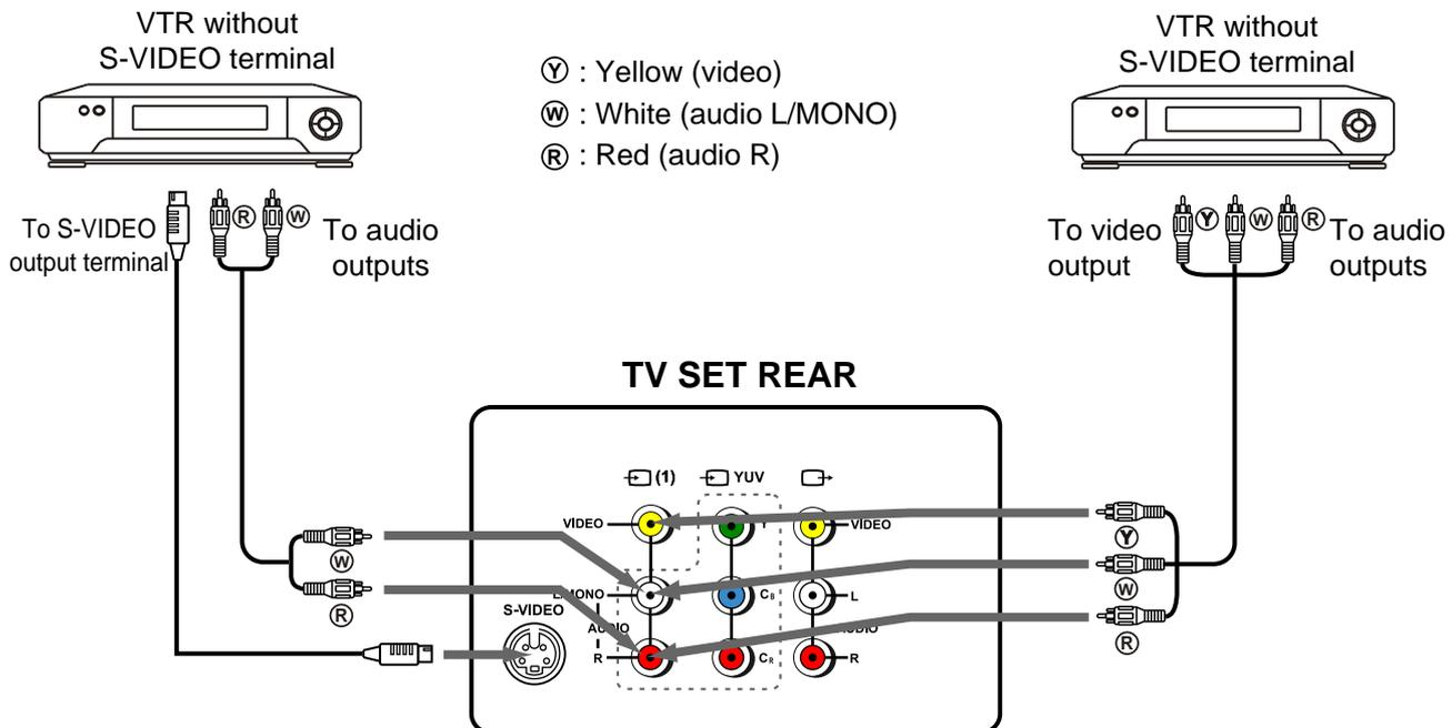
To access the unit connected to these jacks, press **TV/AV** button until **AV1** or **SVHS** appears on the screen.
