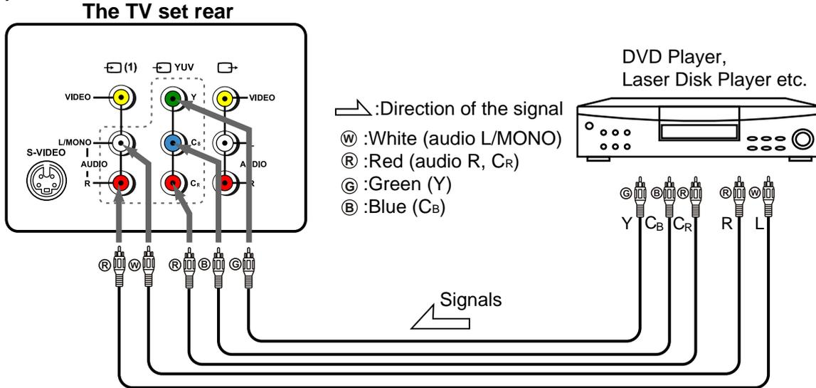
To access the unit connected to these jacks, press **TV/AV** button until **YUV** appears on the screen.
