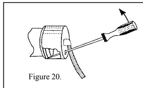
8. Thread the bulb assembly nut until it just touches the fitting body, then finger tighten.
