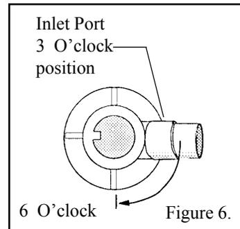
16. Now, from inside the pool, push the bulb assembly and flow director with the red cap/plug in place into the fitting body until the bulb assembly/flow director are nearly flush against the inside pool wall.
