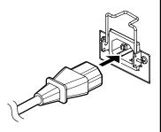
2 Lower the power cord clamp to secure the power cord plug.
