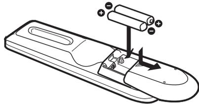
**When you change the batteries, try to complete the task within three minutes. If you take longer than three minutes, the remote control codes for your VCR, DVD, and/or cable box/satellite receiver may have to be reset. See pages 23 - 26.**
