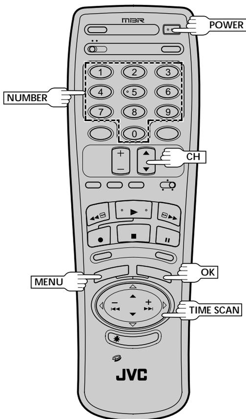
The VCR Plus+ timer programming system eliminates the need to input channel, date, start and stop time data when setting the timer record function. Simply key in the PlusCode number for the TV program you wish to record and the VCR's timer will be automatically programmed. (The PlusCodes are the numbers next to the programs in most TV listings.)
