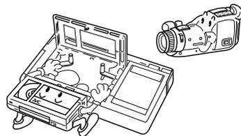
\* Compact VHS camcorder recordings can be played on this video recorder. Simply place the recorded cassette into a VHS Cassette Adapter and it can be used just like any full-sized VHS cassette.
