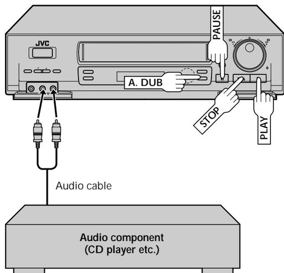
Audio dubbing replaces the normal audio sound of a previously recorded tape with a new soundtrack. Use your VCR as the recorder.
