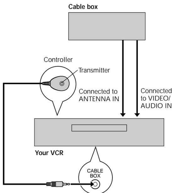
This procedure is required if you receive your TV channels through a cable box (descrambler). The Controller allows the VCR to automatically switch the cable box channel during timer-recording. The Controller is effective for recording shows that have been programmed using VCR Plus+ (☞ pg. 42) or On-Screen Timer Programming (☞ pg. 44).
