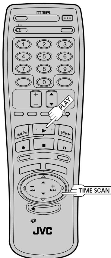
Your VCR is equipped with the TimeScan function. TimeScan allows noise free pictures to be displayed on your TV screen in the forward and reverse search modes. Audio will be played back at normal speed during any of the TimeScan modes (☞ pg. 37). TimeScan allows you to view a program in search mode while listening to the audio.
