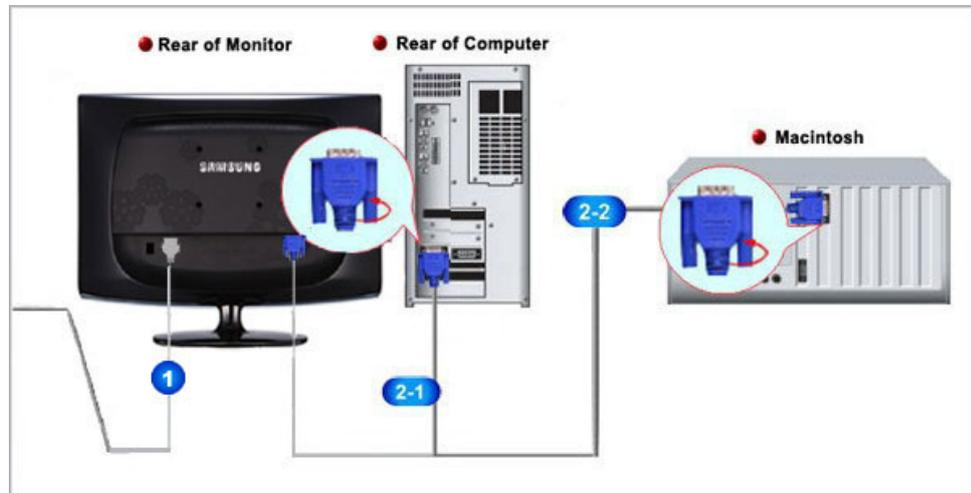
**1** Connect the power cord for your monitor to the power port on the back of the monitor. Plug the power cord for the monitor into a nearby outlet.
