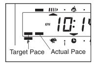
the display. The left column will show one bar, showing that the target pace is 5 mph (8 kph). The right column will show your actual pedaling pace. Adjust your pedaling pace until only one bar appears in the right column. Each time the target pace changes during the program, adjust your pedaling pace to keep both columns at the same height.
