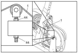
Locate the Drive Belt (1). To tighten the Drive Belt, loosen the bottom M10 Nylon Locknut (44) and then tighten the upper M10 Nylon Locknut (44) slightly; **be careful not to overtighten the Drive Belt.** When the Drive Belt is properly adjusted, tighten the lower M10 Nylon Locknut (44). Then, reattach the left side shield, the flywheel cover, and the left pedal.
