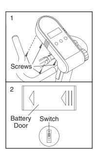
(see drawing 1). Lift the console a few inches and turn it over, being careful not to pull on the wires. Next, look into the hole below the battery door, and locate the small switch (see drawing 2). (Note: It may be necessary to look into the hole and to the left side to find the small switch.) Slide the switch up or down to change the unit of measurement. Reattach the console with the four screws.
