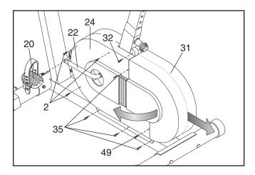
Next, locate the Reed Switch (4). Turn the arms of the Crank (22) until the Magnet (33) is aligned with the Reed Switch. Loosen but do not remove the indicated Screw (35). Slide the Reed Switch slightly closer to or away from the Magnet. Retighten the Screw. Turn the Crank for a moment. Repeat until the console displays correct feedback. When the Reed Switch is correctly adjusted, reattach the left side shield, flywheel cover and left pedal.
