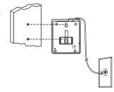
supplied) into each hole, letting the heads extend about <sup>3</sup>/16 inch (5 mm) from the wall. Connect the supplied long modular cord to the phone's line jack. Fit the keyhole slots over the screw heads and slide the phone downward to secure it. Plug the line cord into the telephone line jack.
