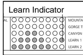
When a custom program is selected, the program display will show a simplified profile of the program. The Time/Laps display will show how long the program will last. **Note: If only three columns of indicators are lit in the program display, refer to HOW TO CREATE A CUSTOM PROGRAM on page 14.**
