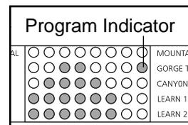
When you select a preset program, the program display will show a simplified profile of the program you have selected. For example, the profile above shows that the intensity of the selected program will increase during the first half of the program, and then decrease during the last half of the program. The Time/Laps display will show how long the program will last.
