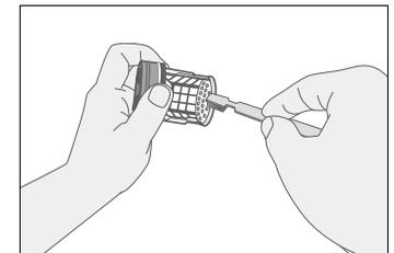
4. Wash any dirt or other material from the filter. Make sure the drain pump propeller behind the filter is not blocked. Replace the filter cap.
