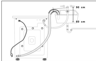
In a sink drain pipe branch
