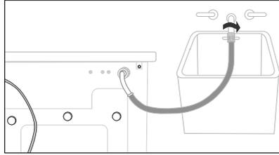
2. Connect the other end of the cold water supply hose to your sink's cold water faucet and tighten it by hand. If necessary, you can reposition the water supply hose at the washing machine end by loosening the fitting, rotating the hose, and retightening the fitting.
