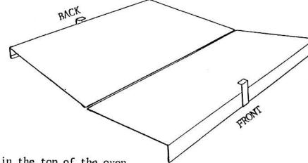
Element Cover must be installed in the top of the oven covering the heater and the fan blade. DO NOT operate without the Element Cover in place.
