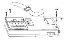
Caution: The BATT TEST button might come off of the front of the TRC-235 when you remove the front cover. If this happens, simply replace it.
