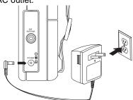
It takes about 20 hours to charge new or fully discharged nickelcadmium batteries. Subsequent charges take about 14 to 16 hours.
