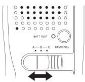
Note: Your TRC-235 comes with Channel 14 crystals installed in channel position A. To use other channels, you must first install crystals in channel positions B and C inside the TRC-235 (see "Adding Crystals" on Page 24).
