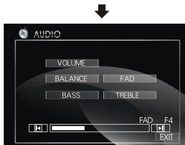
Press **◀** and **▶** to adjust the desired **FAD** level, press **EXIT** to exit this menu.
