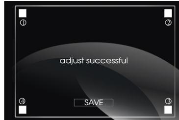
Press ADJUST SCREEN to display the above menu, there are a square button in the top left corner. Press the square button at place ①, then the button will move to place ②, press it at place ②, it will move to place ③, then place ④, press SAVE at last.
